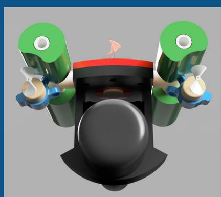
This is the Bathymetric SeaPerch ROV that we designed. The red piece on top would be 3D printed. It would hold the SONAR system below it, the vertical thruster in the middle, and the flotation and horizontal thrusters on either side.
