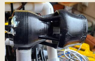
Thrusters are 500 gallons per hour (gph) bilge pump cartridges. Each fitted with 3D printed kort nozzles and removable screens, or "motor covers"
